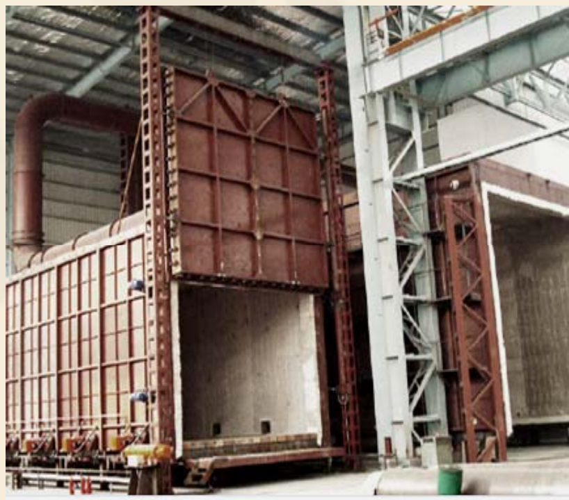
热处理炉 (L24×W6.5×H6.5m)
